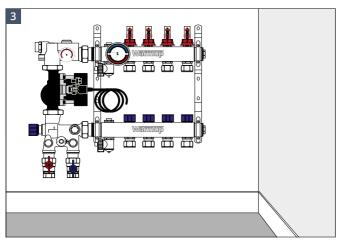
· Identify a suitable location, and mount the manifold.
