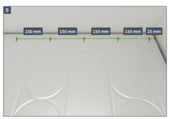
• Screw the Econna-12 panels to the joists using 55 mm wood screws, 25 mm in from each top edge and then at 150 mm centres.
