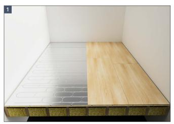
Lay a 6 mm flooring grade plywood in the opposite direction to the Econna-12 panels. The plywood covering should be positioned so that each plywood panel overlaps the tongue and groove edges of the Econna-12 panels by 300 mm.
